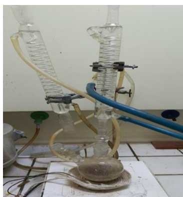
Fig. 1. Reflux system for phthaloylation reaction of chitosan
