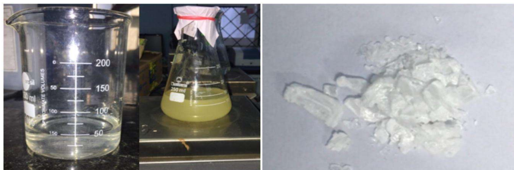
Fig. 1B. Image shows preparation of magnesium oxide nanoparticles from magnesium chloride crystals using Cassia oleoresin
