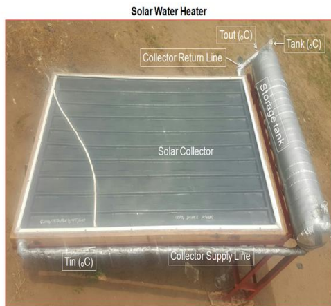
Fig. 3. Picture of the solar collector together with the storage tank
