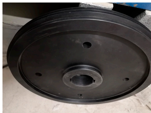
Figure 5. The rotating disk with labyrinth seals and 4 uniformly distributed orifices.
