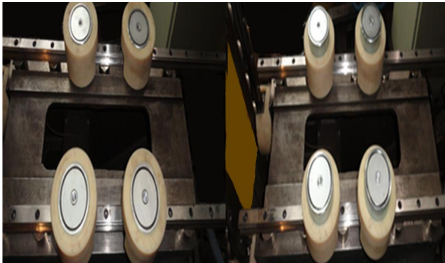
Fig. 6. Carriages, guards and magnetic pots to fulfill knee-saddle assembly
