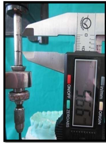
Fig. 14. The distance between two horizontal marks on the vertical arm of the surveyor was measured using a digital vernier caliper
