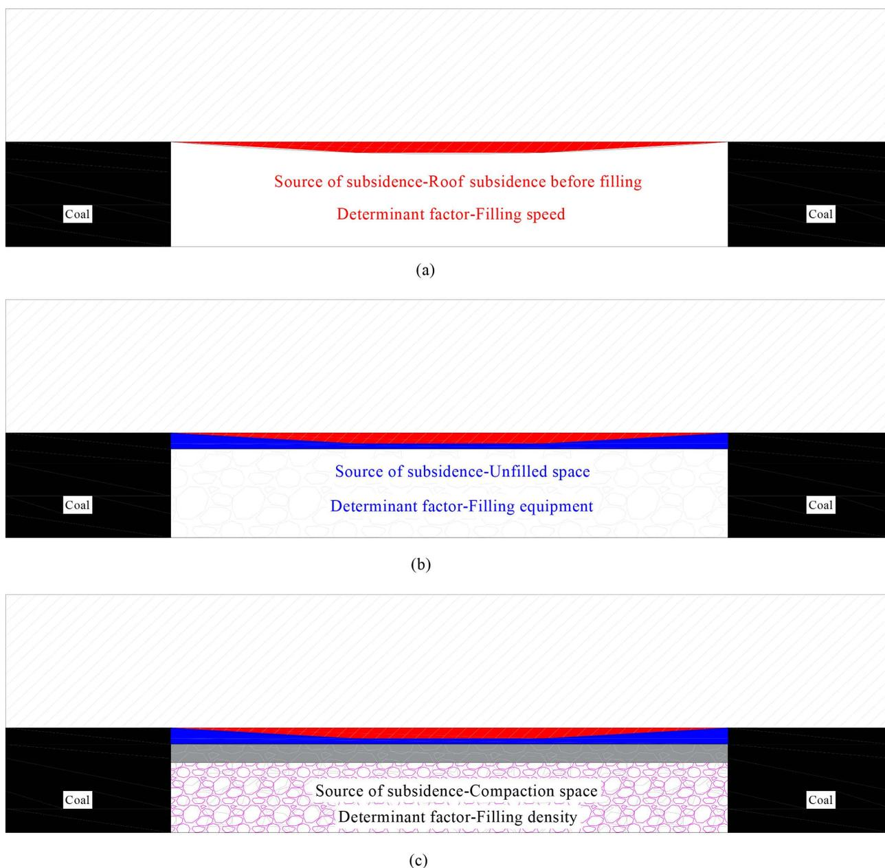
**Figure 6.** Source and control method of gangue filling subsidence at different stages.
