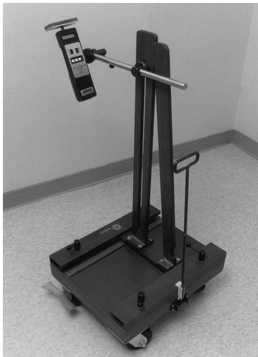
Figure 1. AccuForce II Digital Force Gage attached to a portable steel frame with movable arm and rotating disc and braking mechanism.
