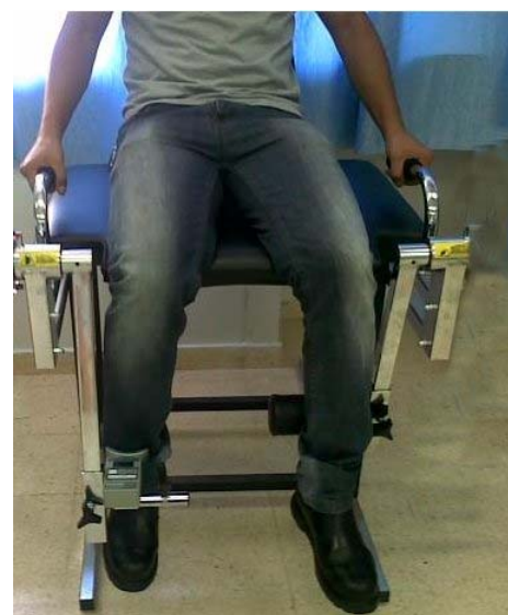
Figure 3. Electronic Pull/push Dynamometer attached to on a new constructed chair.
