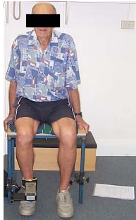
Figure 2. Electronic Pull/push Dynamometer attached to a portable constructed chair to measure muscle strength.
